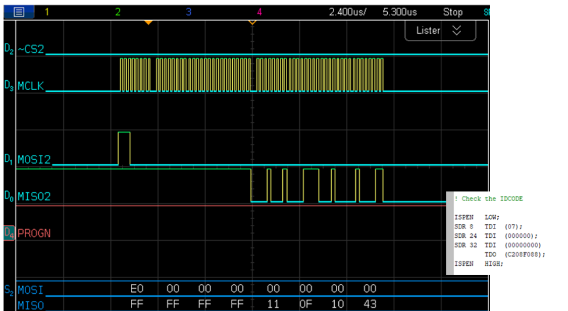
Figure 6.5. READ_ID Command and Device IDCODE Readout
