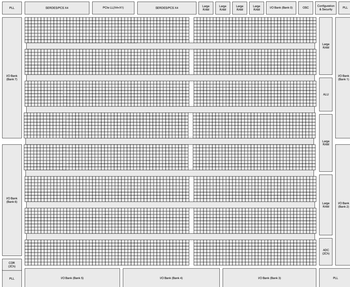
Figure 2.1 Simplified Block Diagram, LFCPNX-100 Device (Top Level)
