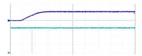
Figure 1: The figure shows the core voltage (blue color) during the powering up sequence and a glitch on the 1553 transmission signal (cyan color).
