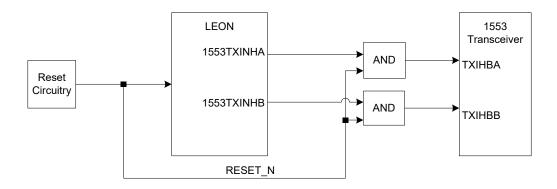
Figure 2: This workaround prevents power up sequence glitches from getting out to the 1553 network
