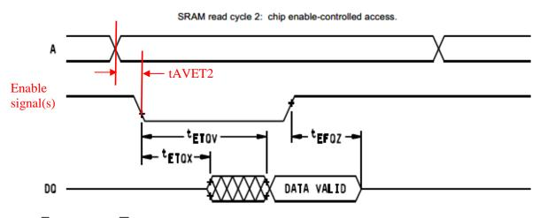
Note:  $\overline{G} \leq V_{IL}(max)$  and  $\overline{W} \geq V_{IH}$  (min).
