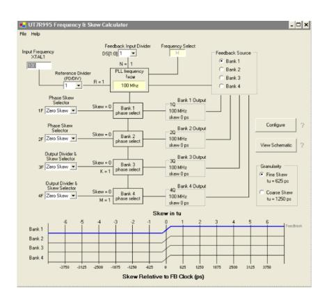
Figure 2. UT7R995/C RadClock™ Calculator and Configuration Tool GUI Example
