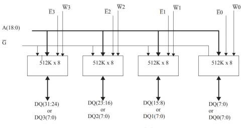
Figure 1. UT9Q512K32E SRAM Block Diagram
