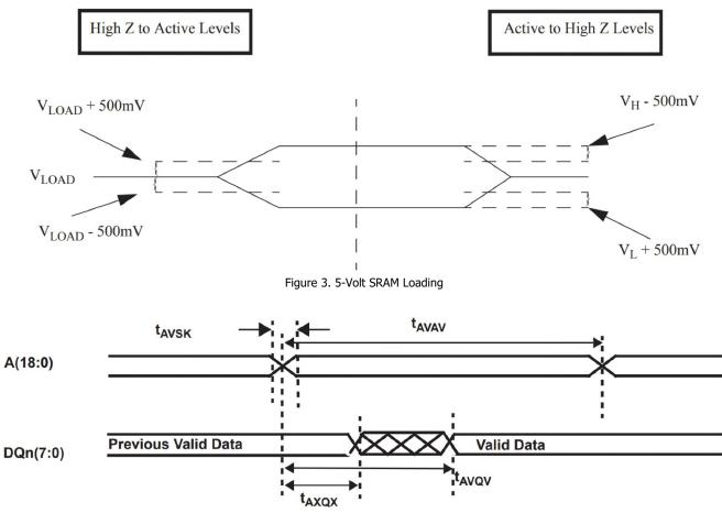
Figure 4a. SRAM Read Cycle 1: Address Access
