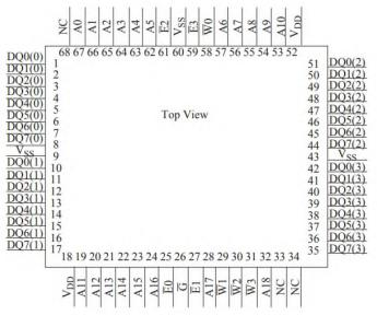
Figure 2. 25ns SRAM Pinout (68)
