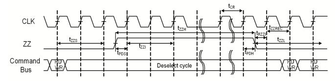
Figure 4. Switching Waveform for SLEEP Mode
