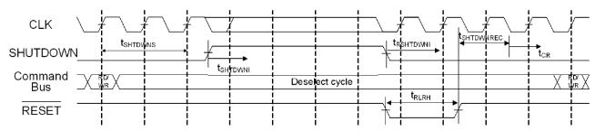
Figure 5. Switching Waveform for SHUTDOWN Mode
