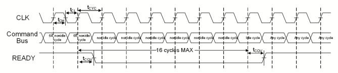
Figure 3. Switching Waveform for Internal Housekeeping
