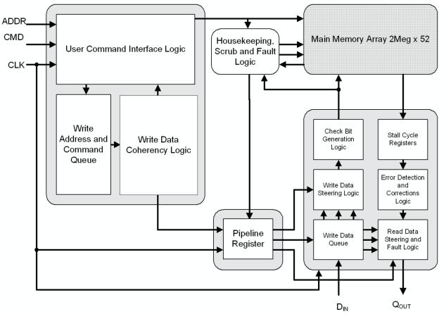
Figure 1. UT8SP2M32 Block Diagram
