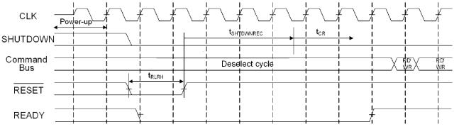
Figure 6. Switching Waveform for Power-Up
