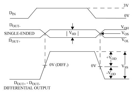
Figure 4. Driver Output Levels
