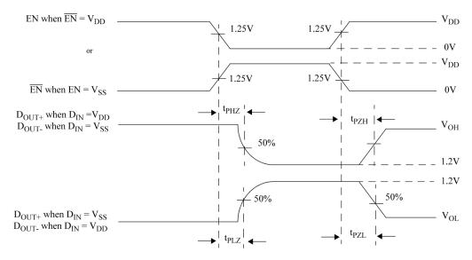
Figure 9. Driver Three-State Delay Waveform
