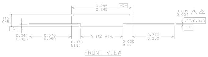
Figure 10. 16-pin Ceramic Flatpack
