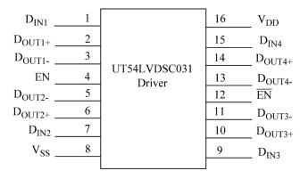
Figure 2. UT54LVDSC031 Pinout
