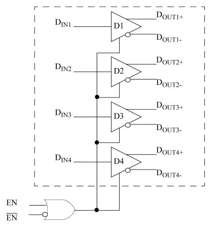
Figure 1. UT54LVDSC031 Quad Driver Block Diagram
