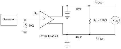
Figure 5. Driver  $V_{\text{OD}}$  and  $V_{\text{OS}}$  Test Circuit or Equivalent Circuit
