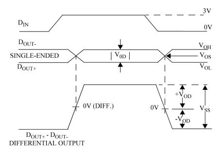
Figure 4. Bus-LVDS Driver Output
