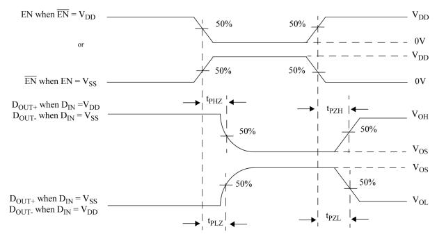
Figure 9. Driver Three-State Delay Waveform
