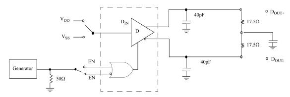
Figure 8. Driver Three-State Delay Test Circuit or Equivalent Circuit
