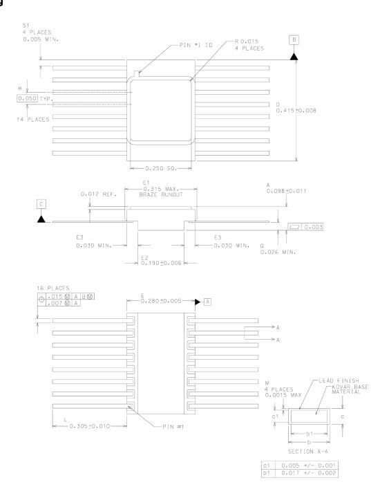
Figure 10. 16-pin Ceramic Flatpack
