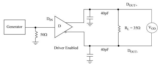
Figure 5. Driver  $V_{\text{OD}}$  and  $V_{\text{OS}}$  Test Circuit or Equivalent Circuit
