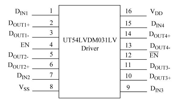
Figure 2. UT54LVDM031LV Pinout
