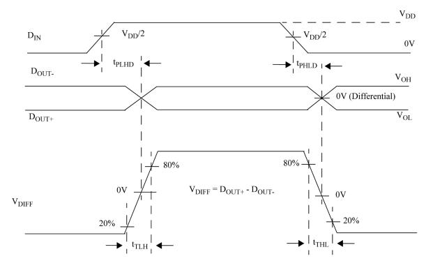
Figure 7. Driver Propagation Delay and Transition Time Waveforms
