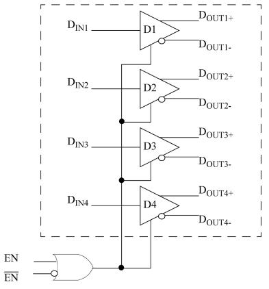
Figure 1. UT54LVDM031LV Bus-LVDS Quad Driver Block Diagram
