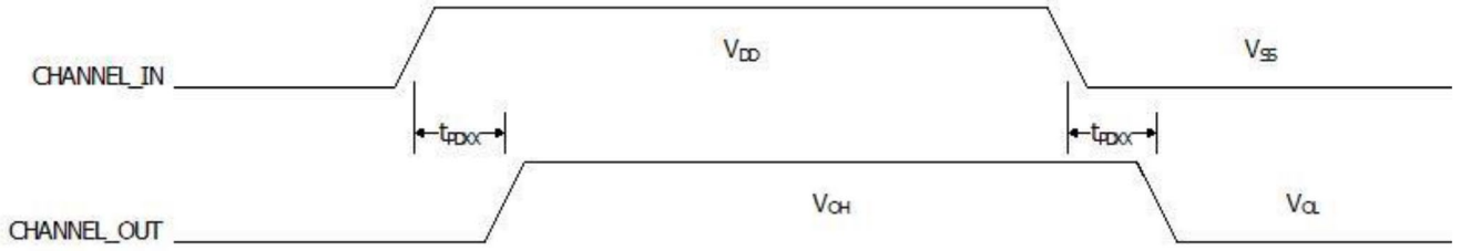
Figure 3: Channel Propagations Delay (/EN = V SS )
