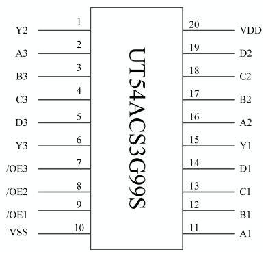
Figure 2: UT54ACS3G99S Pinout Diagram
