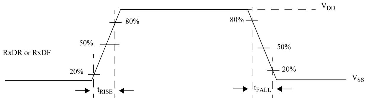
Figure 8. Receiver Output Rise and Fall Times Waveform
