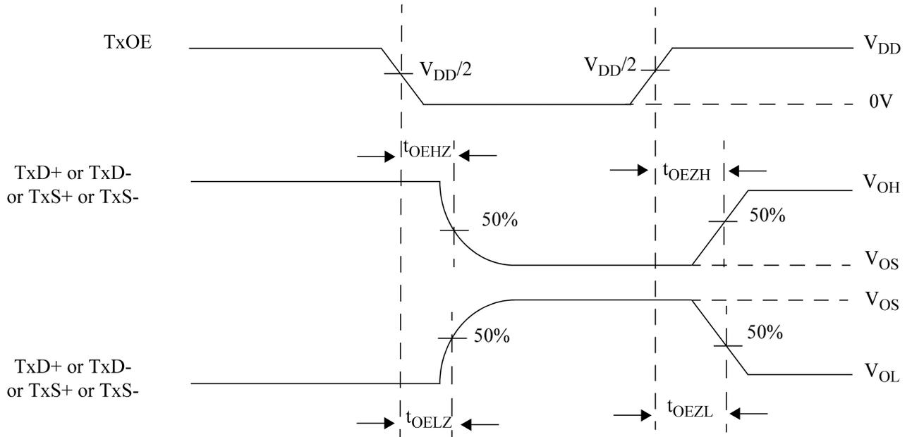
Figure 4. Output Enable to Data Out Timing
