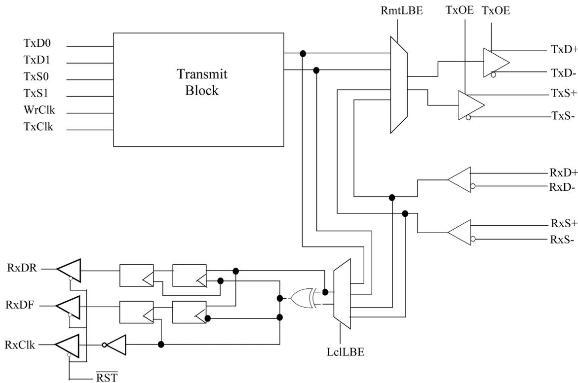
Figure 1. UT200SpWPHY01 SpaceWire PHY Chip Block Diagram
