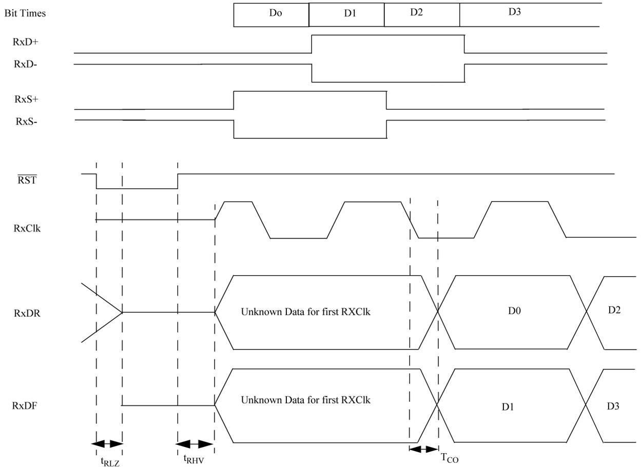
Figure 7. Receiver Output Timing Diagram
