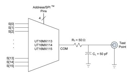
Figure 12. UT16MX113/114/115 Test Circuit
