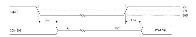
Figure 9: RESET Timing Diagram (Used for UT16MX114/115 only)
