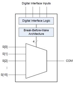
Figure 1. UT16MX113/114/115 Block Diagram
