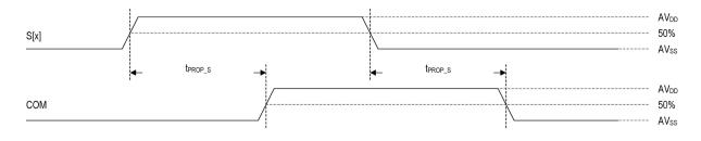
Figure 10. Analog Timing Diagram (Used for UT16MX113/114/115)
