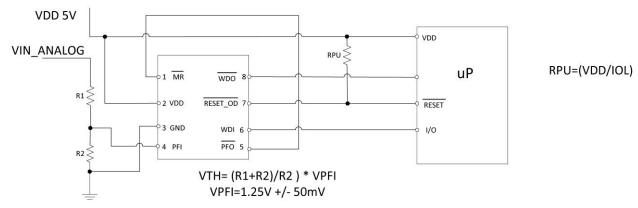
Figure 5. UT01VS50D Under Voltage Monitor and Detection
