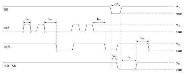
Figure 3. WDI and WDO timing waveforms. Reset externally triggered by MR
