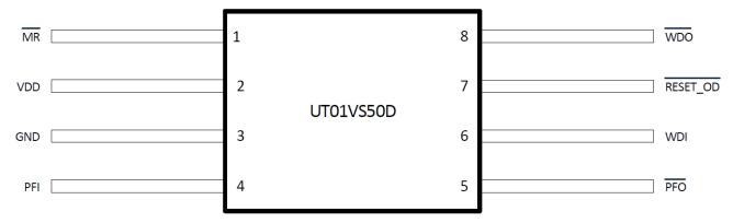
Figure 2. UT01VS50D Pin Configuration
