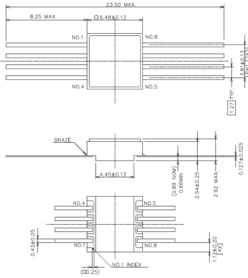
Figure 9. 8-pin Dual-In-Line Flatpack
