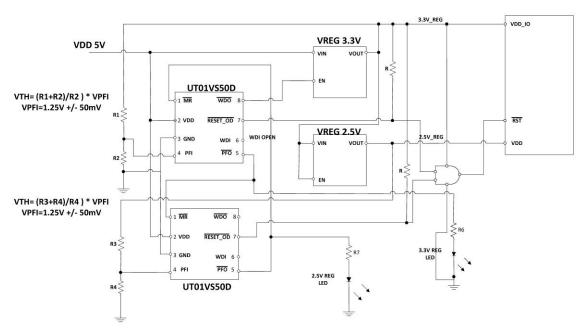
Figure 6. Under Voltage Monitoring and sequencing of 3.3V and 2.5V Power Supplies
