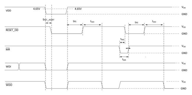
Figure 4. RESET\_OD and WDO are driven low for VDD < 4.65 volts. WDO is driven high when MR is low
