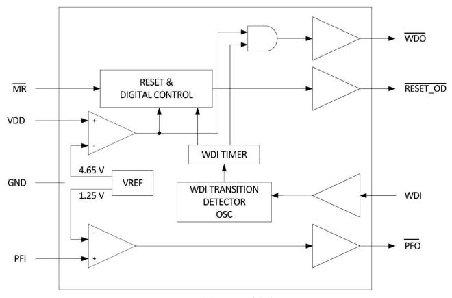
Figure 1. UT01VS50D Functional Block Diagram
