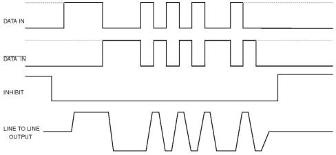
NOTE: DATA and DATA inputs must be complimentary waveforms or 50% duty cycle average, with no delays between them, and must be in the same state during off times (both high or low).
