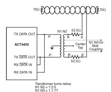
FIGURE 5: TYPICAL TRANSFORMER DIRECT CONNECTION
