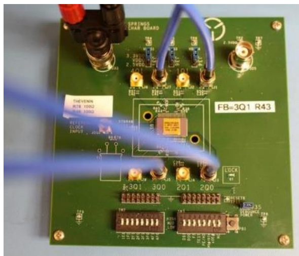
Figure 23: Test Equipment Setup for Sections 4.0 and 4.1 – UT7R995-EVB
