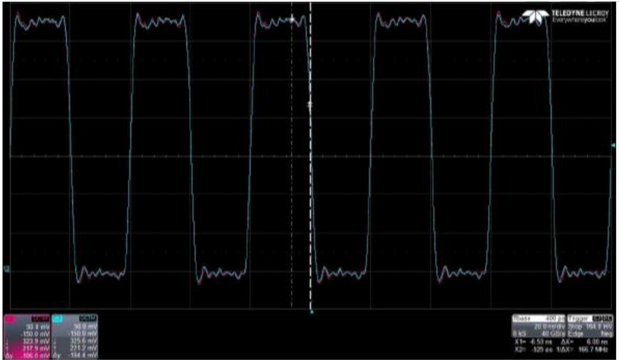
Figure 27: Pre-measurement scope probe calibration using 25MHz system clock
