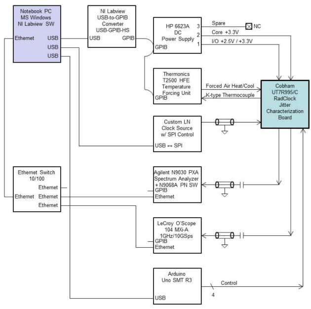
Figure 3.3.1.a: Test Equipment Setup Block Diagram
