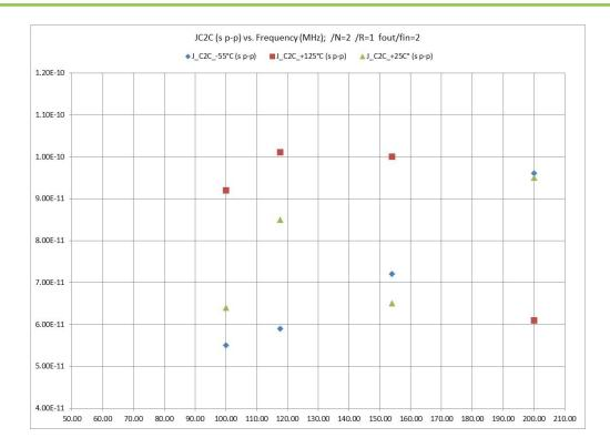
Figure 3.3.2.e: Cycle-to-Cycle (C2C) Jitter (J<sub>C2C</sub>) vs. Output Frequency and PLL Divider Settings: /N=2, /R=1
