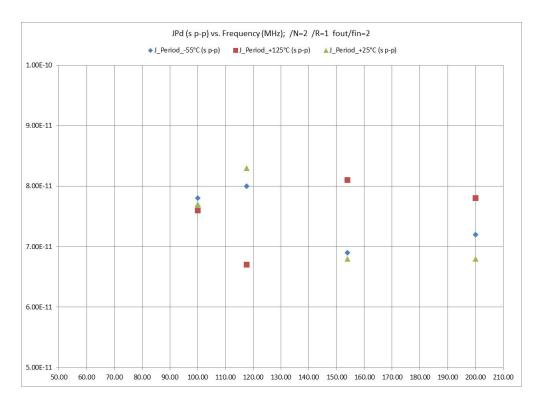
Figure 3.3.3.e: Period Jitter (J<sub>PER</sub>) vs. Output Frequency and PLL Divider Settings: /N=2, /R=1
