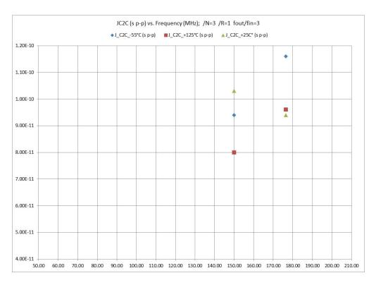
Figure 3.3.2.f: Cycle-to-Cycle (C2C) Jitter (J<sub>C2C</sub>) vs. Output Frequency and PLL Divider Settings: /N=3, /R=1
