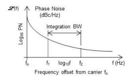
Figure 3.2f: Phase Noise vs. Frequency with Integration BW for J<sub>R</sub> calculations
