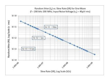
Figure 3.1a: Random Jitter vs. Slew Rate for a Sine Wave Signal (Simulated)
