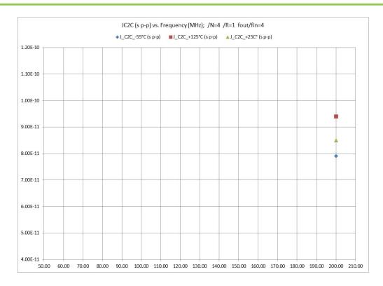
Figure 3.3.2.g: Cycle-to-Cycle (C2C) Jitter ( $J_{C2C}$ ) vs. Output Frequencyand and PLL Divider Settings: /N=4, /R=1
