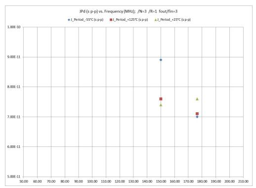
Figure 3.3.3.f: Period Jitter (J<sub>PER</sub>) vs. Output Frequency and PLL Divider Settings: /N=3, /R=1
