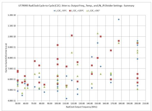
Figure 3.3.2.a: Cycle-to-Cycle (C2C) Jitter (JC2C) vs. Output Frequency and PLL Divider Settings: /N, /R – Summary
