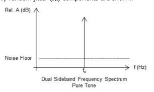
Figure 3.2c: Frequency Spectrum of Single Tone without Phase Noise
