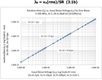
Figure 3.1b: Random Jitter vs. Input Noise Voltage for a Sine Wave Signal (Simulated)
