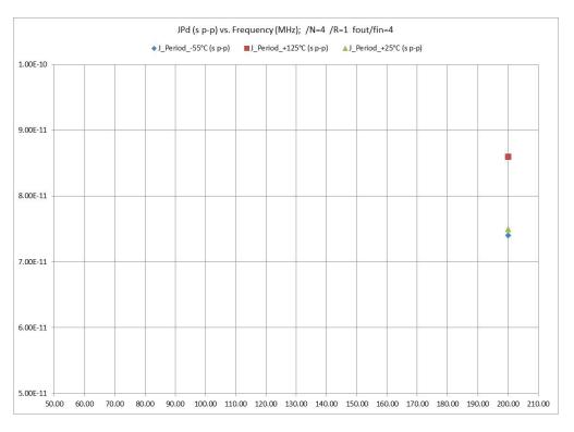
Figure 3.3.3.g: Period Jitter (J<sub>PER</sub>) vs. Output Frequency and PLL Divider Settings: /N=4, /R=1
