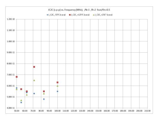
Figure 3.3.2.d: Cycle-to-Cycle (C2C) Jitter (J<sub>C2C</sub>) vs. Output Frequency and PLL Divider Settings: /N=1, /R=2
