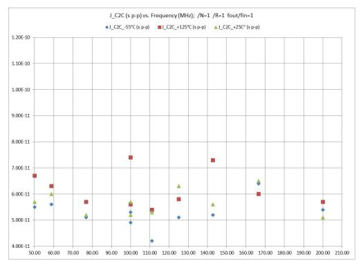
Figure 3.3.2.b: Cycle-to-Cycle (C2C) Jitter (J<sub>C2C</sub>) vs. Output Frequency and PLL Divider Settings: /N=1, /R=1
