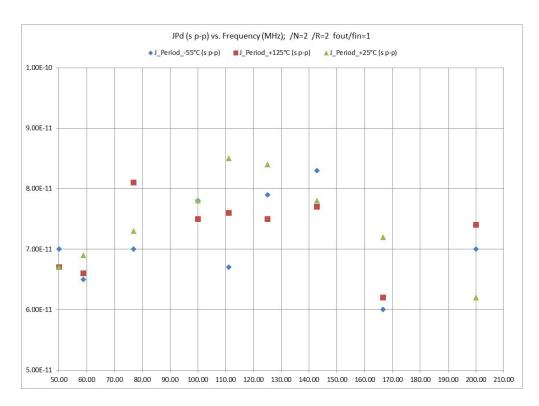
Figure 3.3.3.c: Period Jitter (J<sub>PER</sub>) vs. Output Frequency and PLL Divider Settings: /N=2, /R=2
