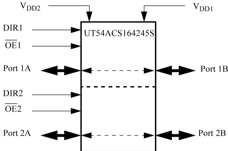
Figure 1. Architectural Block Diagram of the UT54ACS164245S 16-bit (8-bit) Buffer(s)
