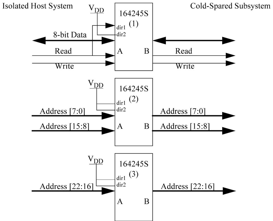
Figure 3. UT54ACS16425S Cold-Sparing Control
