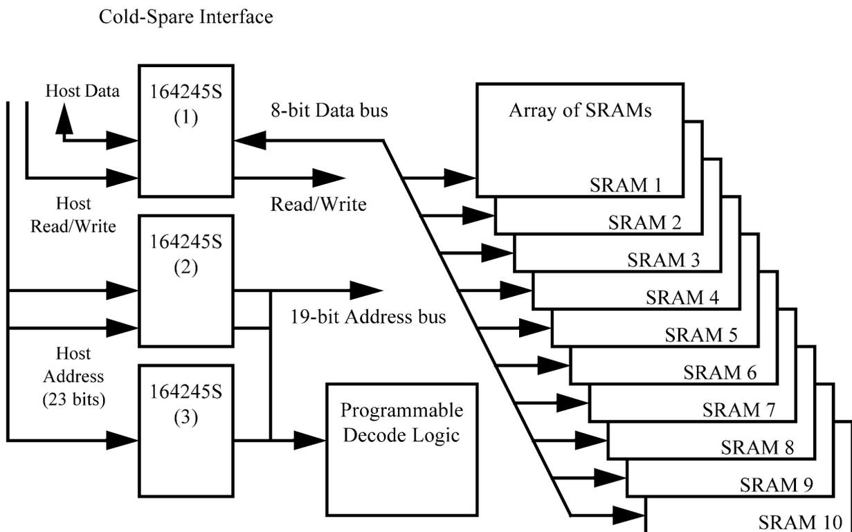
Figure 2. Block Diagram of Cold-Spared Memory Card (Subsystem)
