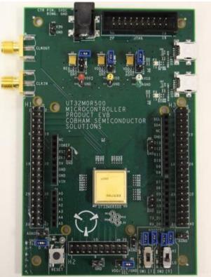
Figure 2: UT32M0R500 Evaluation Board
