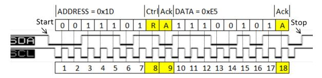
Figure 7: I2C Read Interface Timing Diagram
