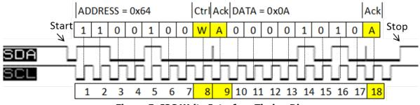
Figure 5: I2C Write Interface Timing Diagram
