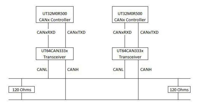
Figure 1: CAN communication system
