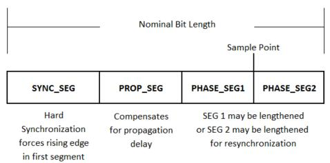
**Figure 8: CAN Input Bit Sample Point**
