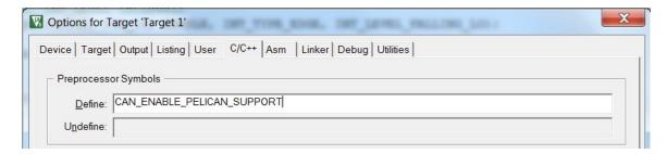
**Figure 9: Extended CAN Support Option**
