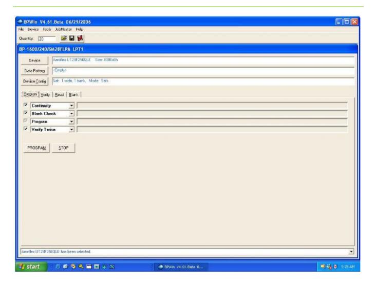
Programming times can vary from 60 to 240 minutes depending on the number of bits that will be programmed. If the device fails verify, discard the part. When programming is complete a security fuse is blown which will disable all test modes used during programming. Trying to program a second block will not work since the tet modes have been disabled.
