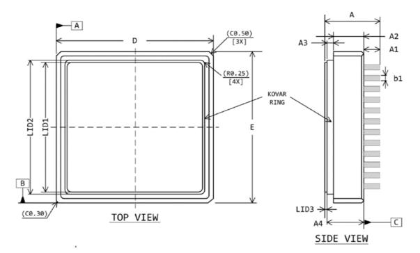
Figure 1. 143-Pin CCGA Package Outline Drawing
