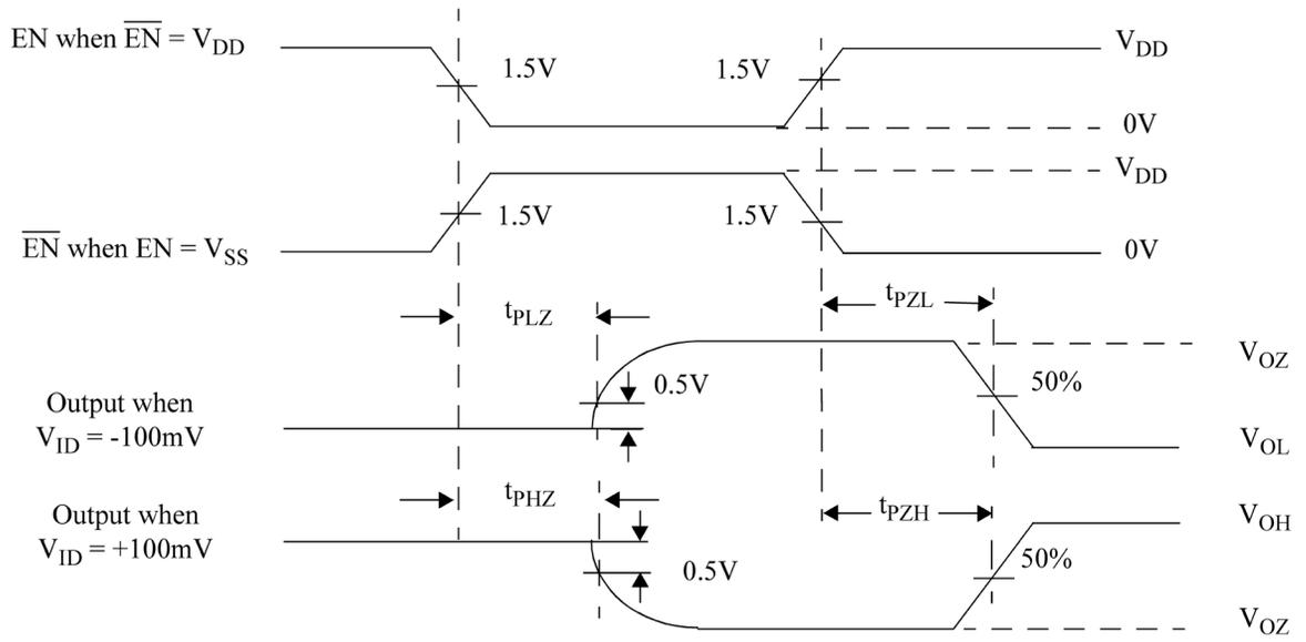
Figure 7. Receiver Three-State Delay Waveform
