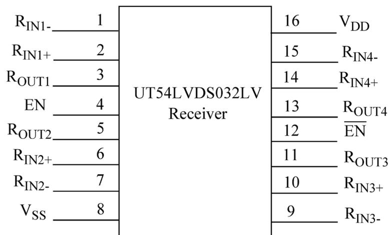
Figure 2. UT54LVDS032LV Pinout
