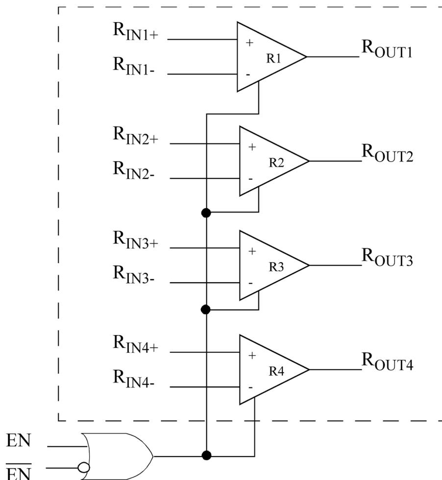
Figure 1. UT54LVDS032LV Quad Driver Block Diagram
